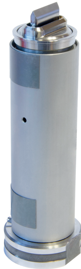
Fig. 2. FDU Midi (open version): This nozzle was used in this project with Walther Faltsysteme © FDU Hotrunner
